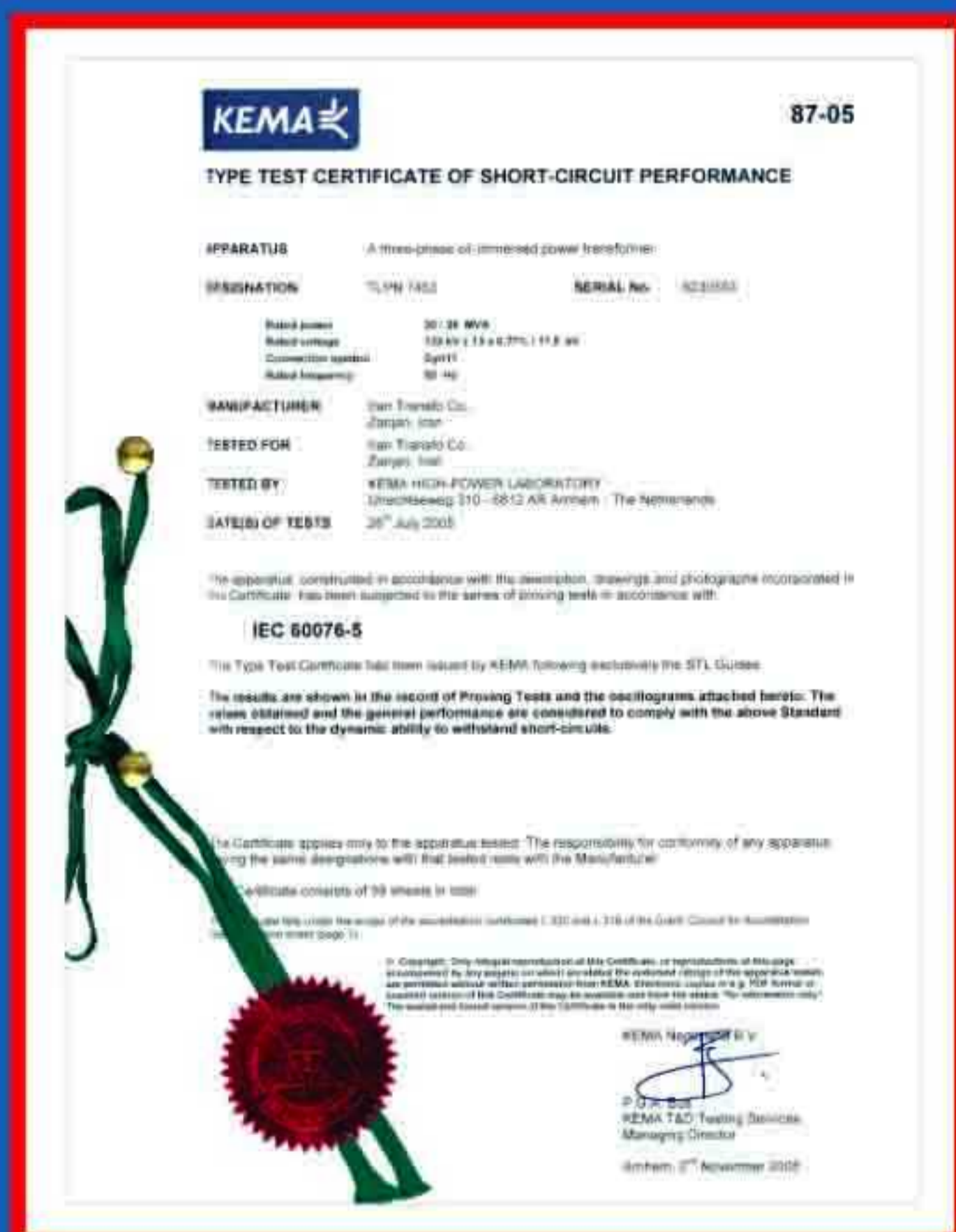
Certificate of short circuit test 26 MVA - 132/11.5kV
