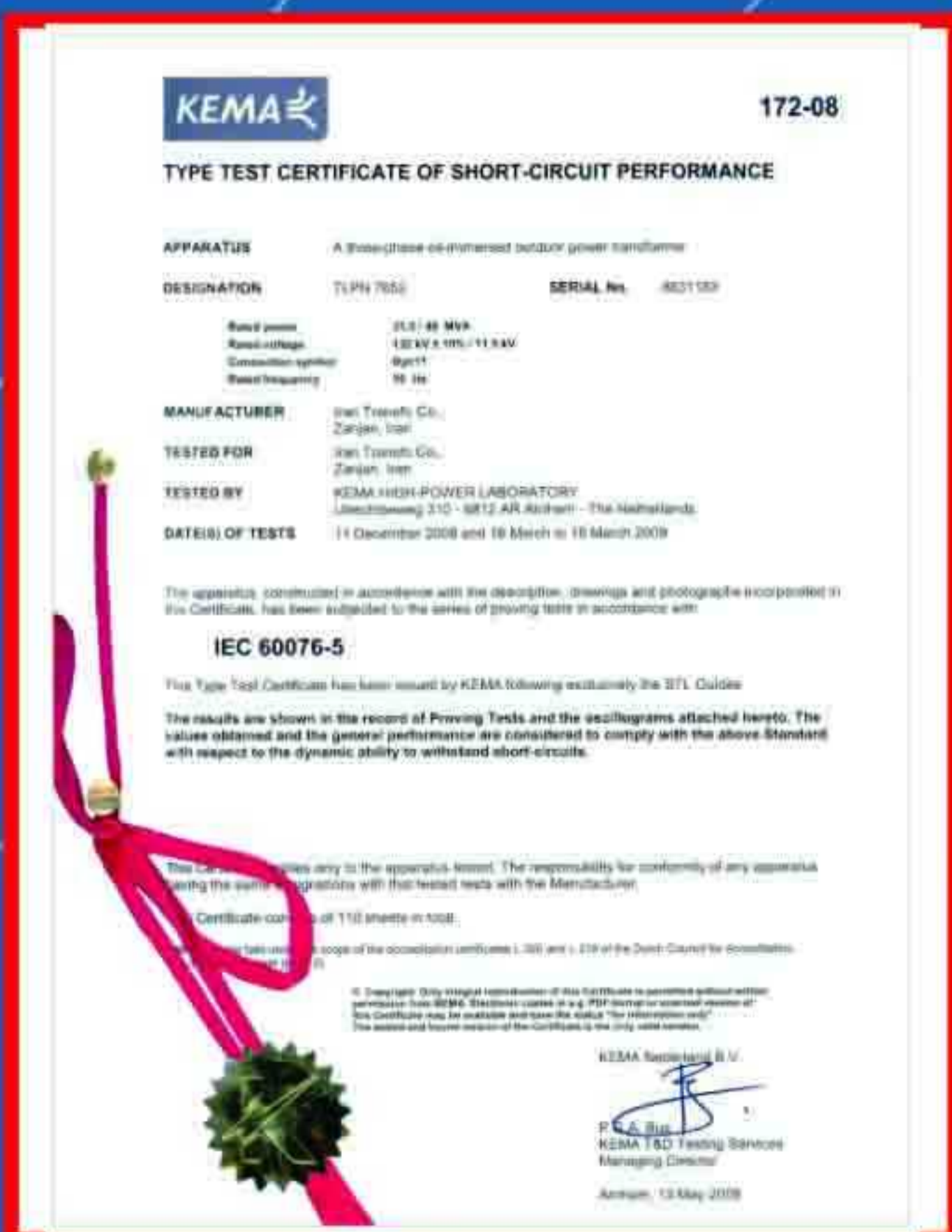
Certificate of short circuit test 40 MVA - 132/11.5kV
